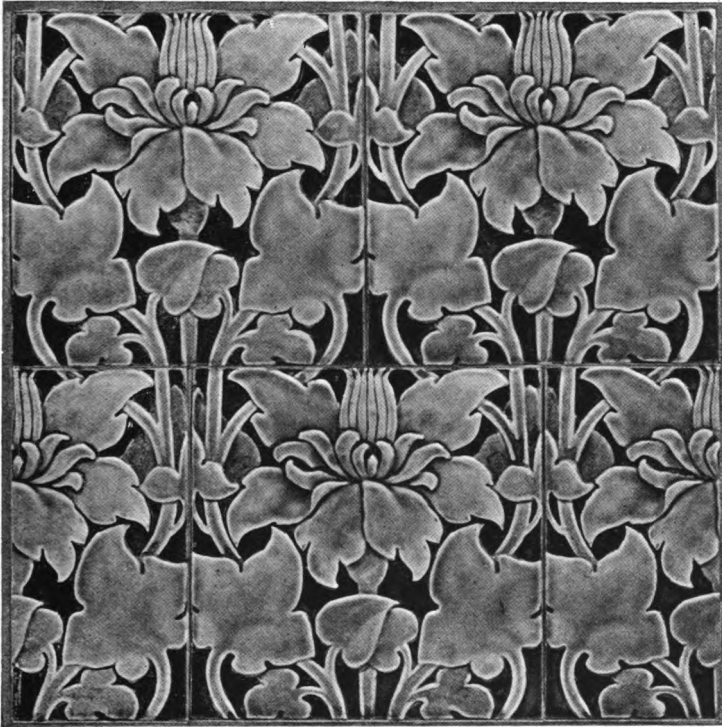
158. SIX-INCH TILE DESIGNED TO BE FIXED BRICKWISE.
